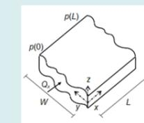
The pressure gradient is transverse to the aperture variability
